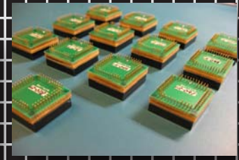
CZT Modules for a Large Area Gamma Radiation Detector Array
